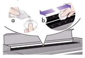
7 Dry the glass completely using a separate clean, dry lint-free cloth like the one provided with the maintenance kit.
