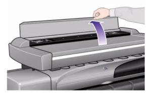
4 Remove the Guide Plate by pressing down on the Plate as you pull the left and right sliders towards the scanner's center until the metal safety buttons on each side of the scanner, pop up.
