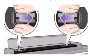
**5** Use the two handles to lift out the Guide Plate.
