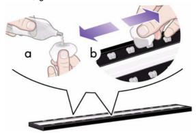
11 Dry the platen and rollers completely using a separate clean, dry lint-free cloth.
