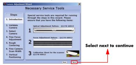
5 The next 4 screens contain information on how to perform the camera Adjustment correctly. Select next after reading each screen.
