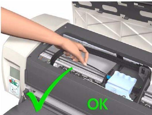
Correct: move using the belt.
