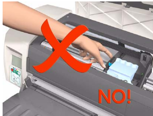
Incorrect: never move using Carriage Assembly.
