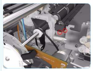
**17.** Remove 2 T-10 screws that secure the bracket on the left hand side of the Printer.
