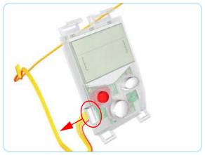
**4.** Disconnect the cable from the Front Panel and remove from the Printer.
