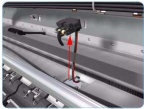
**9.** Remove the OOPS Sensor (including the cable) from the Printer.
