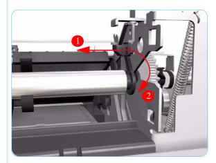
**23.** Release the locking mechanism that secures the Pick Assembly on the right hand side of the printer (looking from the rear).
