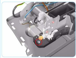
**8.** Remove 1 T-10 screw from the Ramp Motor Assembly.
