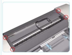
**4.** Remove 4 T-10 screws that secure the Center Cover to the Printer.
