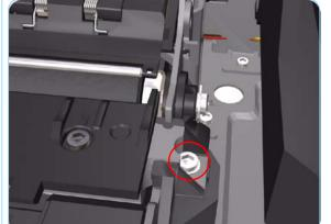
**6.** Remove 1 T-8 screw and washer that secure the Pivot Assembly on the right hand side of the Printer.
