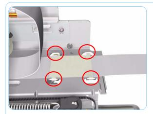
**10.** Release the Trailing Cable from the Chassis.
