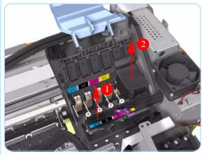
**8.** Lift up the Tube Crane to release the PH Cover from the Carriage Assembly and remove from the Printer.
