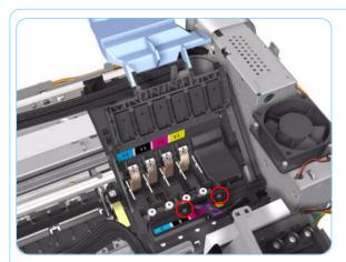
**7.** Open the Printhead Cover and remove 2 T-8 screws that secure the Tube Crane to the Carriage Assembly.
