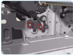
**13.** Remove 2 T-10 screws that secure the Pivot Assembly Support on the right hand side of the Printer.
