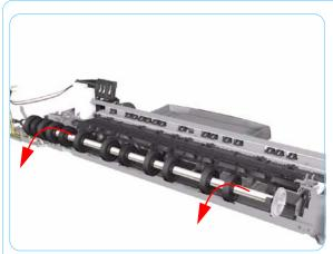
**25.** Raise the locks so that they are aligned with the cutouts and lift out the Pick Assembly from the Printer.
