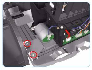
**8.** Remove 2 T-10 screws that secure the lnk Supply Station.
