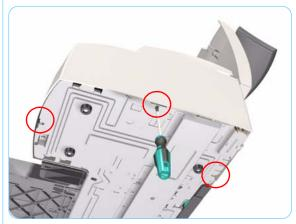
**6.** Release the clips that secure the Right End Cover to the Printer (use a flat-blade screwdriver if necessary).
