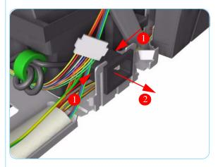
5. Remove the Power Supply from the Printer.
