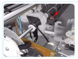
**18.** Remove the Bracket from the Printer.
