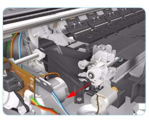
**6.** Remove 1 T-10 screw that secures the Spring Idler. Remove the Spring Idler from the Printer.
