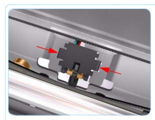
**8.** Press the OOPS Sensor clips inwards to release it.
