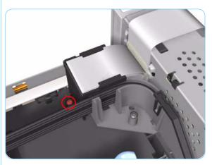
**5.** Remove 1 T-10 screw that secures the Trailing Cable Support to the Carriage Assembly. Release the Trailing Cable Support from the Carriage Assembly.
