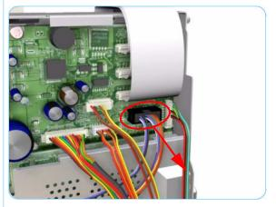
**6.** Disconnect the Ink Supply Station Cable from the Main PCA.
