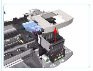
5. Remove the ISS Cover from the Printer.
