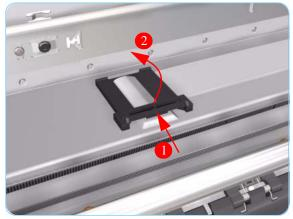
Release the Trailing Cable Clip from the Chassis.
