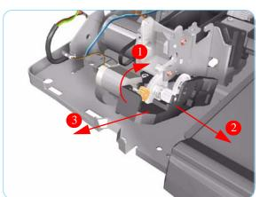
**9.** Remove the Ramp Motor Assembly from the Printer.
