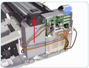
**10.** Slide the Power Supply Unit upwards to release it from the Electronics Module.
