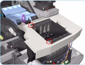
**4.** Remove 2 screws that secure the ISS Cover to the Ink Supply Station.
