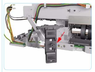
**21.** Remove the Rear Right Trim Bracket from the Printer.
