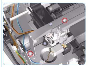
**5.** Remove 2 T-10 screws that secure the Starwheel Assembly to the left hand side of the printer.
