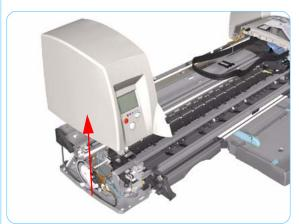
**7.** Remove the Left End Cover from the Printer.
