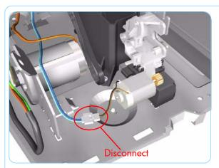
**7.** Disconnect the Ramp Motor cable.
