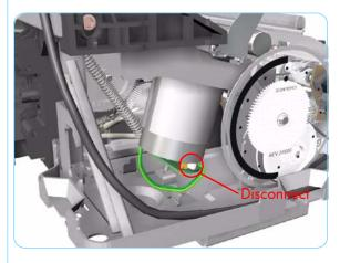
5. Release the Belt from the Carriage Motor by pushing in the Turnaround Assembly (right hand side of the printer) and at the same time releasing the Belt from the Motor on the left hand side of the printer.
