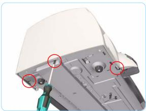
**6.** Release the clips that secure the Left End Cover to the Printer (use a flat-blade screwdriver if necessary).
