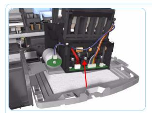
**10.** Remove the Ink Supply Station from the Printer.
