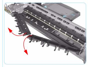
**4.** Remove both pieces of the Inner Paper Guide from the Printer.
