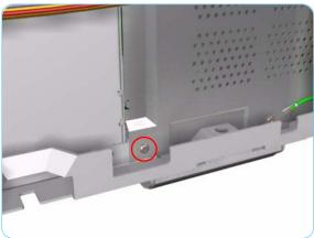
**5.** Remove 1 T-10 screw securing the Plastic Cover. Remove the Plastic Cover from the Printer.
