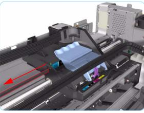
**6.** Gently slide out the Encoder Strip through the Carriage Assembly and remove from the Printer.
