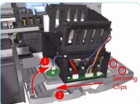
**9.** Rotate the Ink Supply Station upwards and then to the left to release it from the securing clips.
