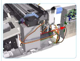
**11.** Remove the Electronics Module from the Printer.
