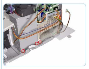
**5.** Remove 3 T-10 screws that secure the Electronics Module and the Power Supply Unit to the Printer.
