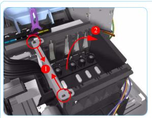
**7.** Release the Tubes Bracket from the Ink Supply Station by pushing the clips inwards and lifting up the Bracket.
