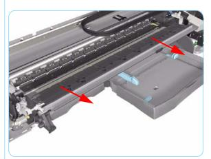
**9.** Slide out the complete Print Platen Assembly.
