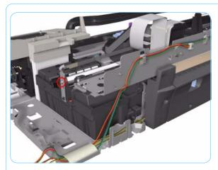
**10.** Remove 1 T-10 screw that secures the Encoder Strip Holder on the right hand side of the Printer.
