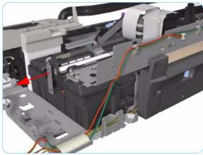
**11.** Remove the Encoder Strip Holder from the Printer.
