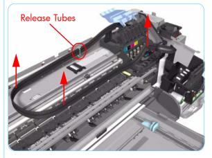
**9.** Release the Ink Supply Tubes from the Raceway Holder and remove from the Printer.
