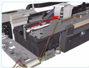
**8.** Move the Carriage Assembly out of the Service Station.
