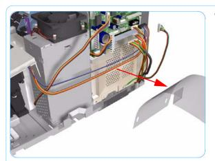
**6.** Remove the Plastic Cover from the Printer.
