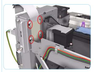
**8.** Release the plastic sheet that secures the Trailing Cable to the back of the Electronics Module.
