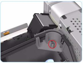
**6.** Remove 1 T-10 screw that secures the Tube Crane to the Carriage Assembly.
