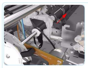
**18.** Remove the Bracket from the Printer.
