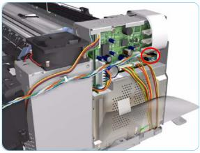
**4.** Disconnect the Ink Supply Station Cable from the Main PCA.
