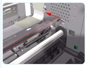
**5.** Release the Encoder Strip from the right hand side of the Printer.
