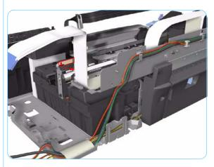
**9.** Release the Encoder Strip from the Encoder Strip Holder.
