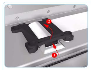
**10.** Release the Trailing Cable Clip from the Chassis.
