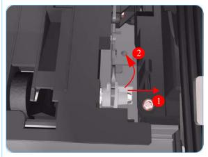
**8.** Release the locking mechanism from the right hand side of the Printer.
