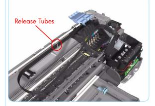
**7.** Release the Ink Supply Tubes from the Raceway Holder.
