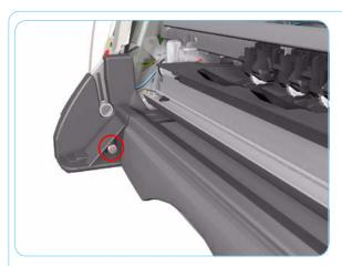
**5.** Remove 1 T-10 screw from the Left Side Bracket.
