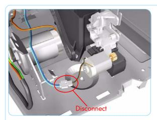
**7.** Disconnect the Ramp Motor cable.
