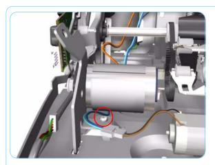
**12.** Remove 1 T-10 screw that secures the Paper-Axis Motor Mount.
