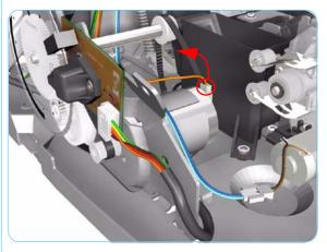
**4.** Disconnect the Paper-Axis Motor cable.
