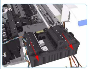
12. Slide the Service Station out of the Printer.
