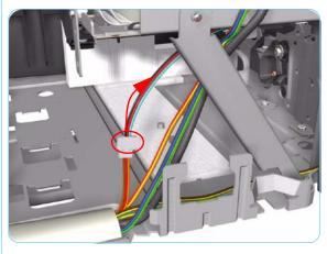
**7.** Remove the Spring that secures the OOPS Sensor.
