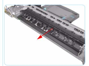
**14.** Remove both pieces of the Inner Paper Guide from the Printer.
