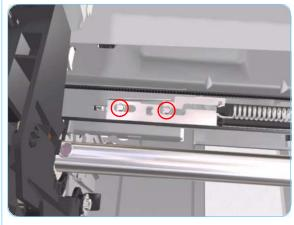
**11.** Remove 2 T-10 screws that secure the Turnaround Stopper. Remove the Turnaround Stopper from the Printer.
