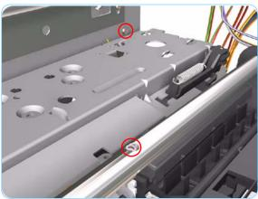
**17.** Remove 2 screws that secure the Hanger Assembly on the right hand side of the Printer.
