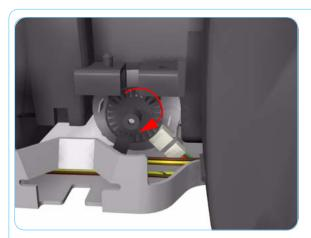
**7.** Uncap the Carriage Assembly by turning the Service Station Motor clockwise.
