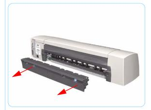
**2.** Remove the Cleanout Assembly from the Printer.
