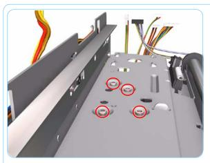
**16.** Remove 4 screws that secure the Hanger Assembly on the right hand side of the Printer.
