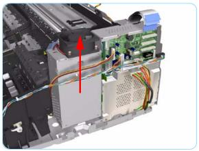
**10.** Slide the Power Supply Unit upwards to release it from the Electronics Module.
