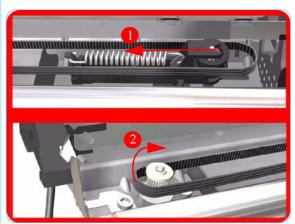
**12.** Release the Belt from the Carriage Motor by pushing in the Turnaround Assembly (right hand side of the printer) and at the same time releasing the Belt from the Motor on the left hand side of the printer.
