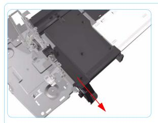
19. Slide the Left Bracket out of the Printer.
