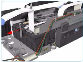
**11.** Remove the Encoder Strip Holder from the Printer.
