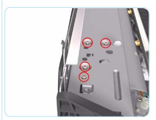
**12.** Remove 1 screw that secures the Hanger Assembly on the left hand side of the Printer.
