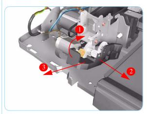
**9.** Remove the Ramp Motor Assembly from the Printer.
