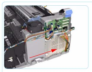
Slide out the Electronics Module and the Power Supply Unit (as one assembly) to the right.
