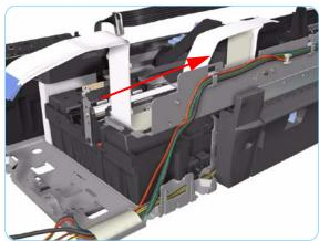
**8.** Move the Carriage Assembly out of the Service Station.
