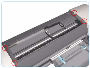
**4.** Remove 4 T-10 screws that secure the Center Cover to the Printer.
