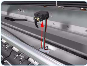
**9.** Remove the OOPS Sensor (including the cable) from the Printer.
