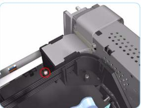
**4.** Remove 1 T-10 screw that secures the Trailing Cable Support to the Carriage Assembly. Release the Trailing Cable Support from the Carriage Assembly.
