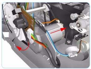
**5.** Release the belt from the Paper-Axis Motor. Remove the Paper-Axis Motor Assembly from the Printer.
