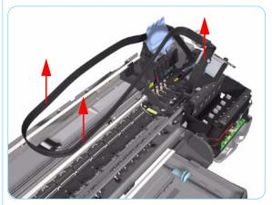
**8.** Release the Ink Supply Tubes from the Carriage Assembly and remove from the Printer.
