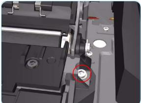
7. Remove the Pivot Assembly from the Printer.
