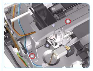
**5.** Remove 2 T-10 screws that secure the Starwheel Assembly to the left hand side of the printer.
