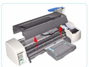
**7.** Remove the Center Cover from the Printer.
