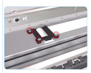
Release the Trailing Cable Clip from the Chassis.
