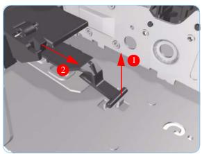
**22.** Remove the Bypass Platen Actuator from the Printer.
