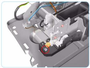
**8.** Remove 1 T-10 screw from the Ramp Motor Assembly.
