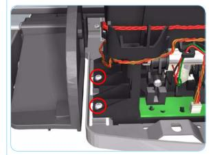
**7.** Remove 2 T-10 screws that secure the lnk Supply Station.
