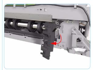
**15.** Remove the Rear Left Trim Bracket from the Printer.
