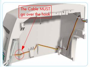
When installing the Front Panel, make sure you route the cable as shown:
