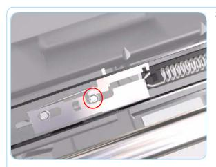
**3.** Insert the 2nd screw (right) and tighten it. As you tighten the screw you should notice that the slot in the Stopper will rise away from the Turnaround Assembly.
