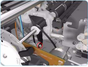
**16.** Remove 1 T-10 screw and nut that secures the Feed-Roller Support on the left hand side of the Printer.
