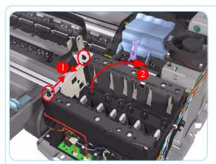
**6.** Release the Tubes Bracket from the Ink Supply Station by pushing the clips inwards and lifting up the Bracket.
