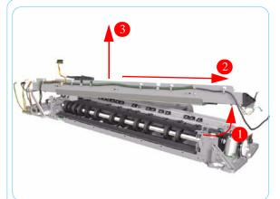
**22.** Remove the Hanger Assembly from the Printer.
