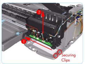
**8.** Move the Ink Supply Station to the left to release it from the securing clips and then upwards out of the Printer.
