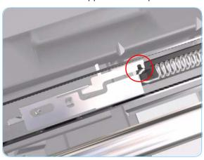
Place the Turnaround Stopper in to position and locate the slot in the Stopper on to the Turnaround Assembly. This step is very important since it will determine the space between the Stopper and the Turnaround Assembly.
