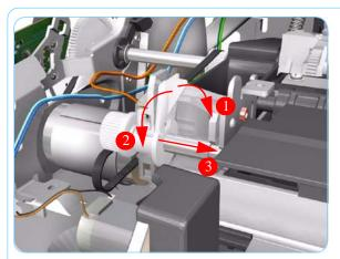
**7.** Release the locking mechanism from the left hand side of the Printer.
