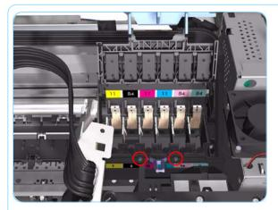
**6.** Open the Printhead Cover and remove 2 T-8 screws that secure the Tube Crane to the Carriage Assembly.
