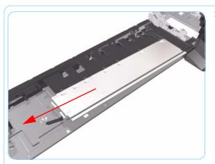
**22.** Slide the Bypass Platen to the left and remove from the Printer.
