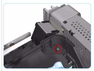
**5.** Remove 1 T-10 screw that secures the Tube Crane to the Carriage Assembly.
