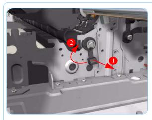
**15.** Release the locking mechanism from the right hand side of the Printer.
