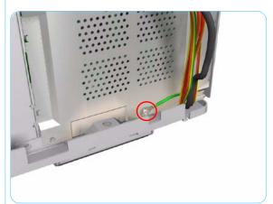
**7.** Remove 1 T-10 screw that secures the Electronics Module.
