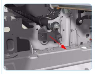
**14.** Remove the Pivot Assembly Support from the Printer.
