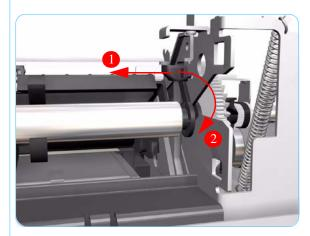
**23.** Release the locking mechanism that secures the Pick Assembly on the right hand side of the printer (looking from the rear).
