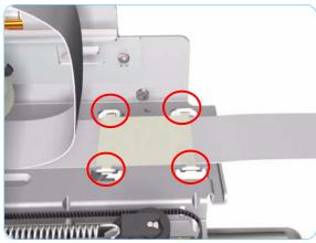
**11.** Release the Trailing Cable from the Chassis.
