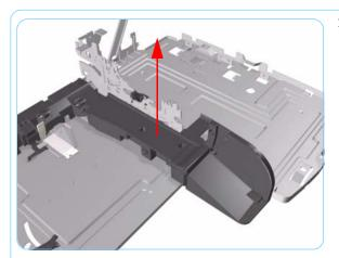
**20.** Lift the Right Bracket out of the Printer.
