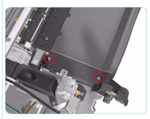
**6.** Remove the Front Left Bracket from the Printer.
