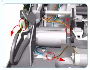
**13.** Disconnect the Paper-Axis, Encoder and Ramp Motor cables.
