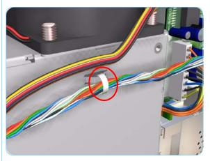
**5.** Cut the Plastic Tie that secures the Ink Supply Station Cable to the Power Supply Unit.
