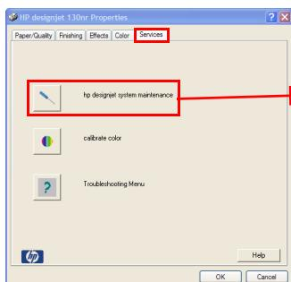
Launch system maintenance tool via the hp driver
