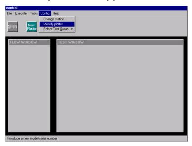
**6** A box will appear prompting you to select the Printer Model and to type in the Printer Serial Number.
