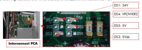
5V - Comes from the PSU after the fuse on Interconnect PCA. Used to power On Front Panel and some Interconnect Electronics. Should be ON at the same time as Blue Power Switch LED.
