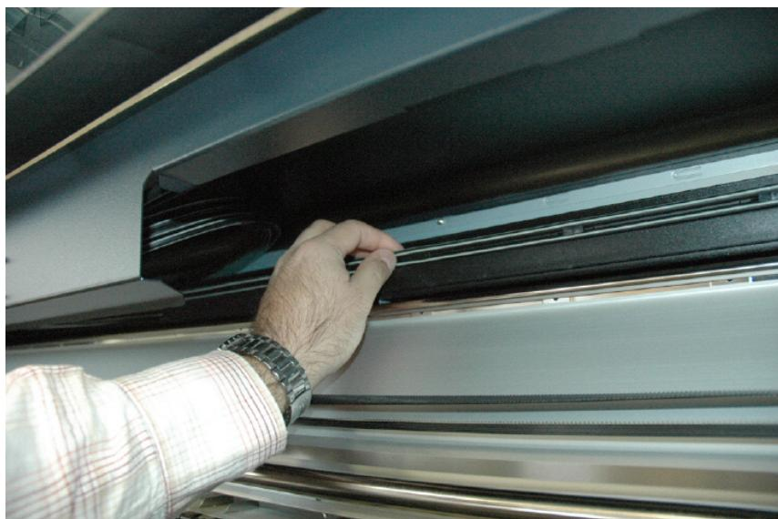
Ink tubes are placed back in its tube guide, as shown in the picture above.
