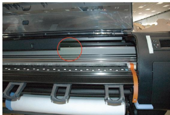
The carton pad has a slot where the metal bracket must be inserted.
