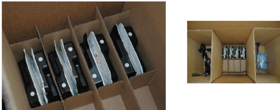
Complete the boxes with the ink supplies, print-head cleaner, cables, 3" core adaptor, CD, etc., and place them over the printer box.
