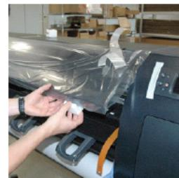
Once the foams are inserted, you can secure the window with 2 adhesive tape stripes.
