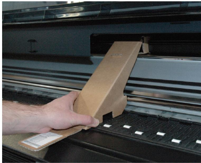
While is being placed, please, ensure the metal gets into the carton slot. This will prevent the carton to move during transportation.
