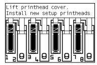
**6** Once all the Setup Printheads are installed, the following message will appear on the front panel. Close the carriage cover and close the window.
