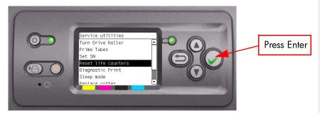
2 You will be given an option to either reset the Life Counter for ALL the parts related to a Preventive Maintenance Kit (PMK) or to just reset the Life Counter for a particular part:
