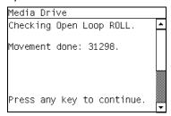
Check that the movement done is more than 100 encoder units (in absolute value). If the movement done is less than 100 encoder units then open the Window and check for any visible obstacles restricting the movement of the Drive Roller or the Overdrive Assembly. In this case, press any key to finish the test.
