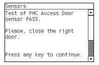
If the PHC Access Door Sensor fails the test, the Front Panel will display **System Error Code 51.1:10**. For more information on troubleshooting this error code, refer to Page 2-15. Check also **System Error Code 07:10** (refer to Page 2-6).
