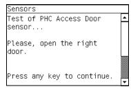
**8** If the PHC Access Door Sensor passes the test, the following message is displayed on the Front Panel. Close the PHC Access Door and press any key to continue.
