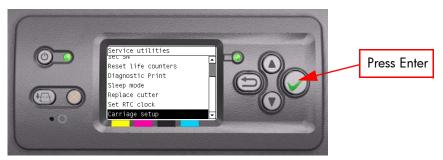
When the following message appears on the front panel, you must select whether you would like to continue with the Carriage Setup by pressing Enter. Press Back or Cancel to exit the utility.
