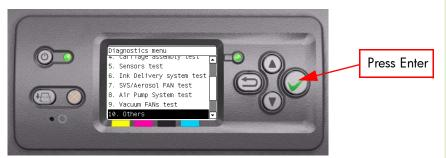
2 In the Others submenu, scroll to "10.1 Bag Broken Recovery" and press **Enter**.
