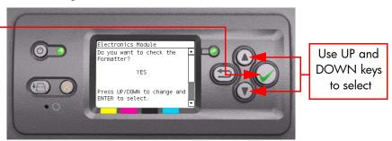
3 If you select **Yes**, the printer will get the CPU information and display the information on the Front Panel. Press any key to continue the test:
