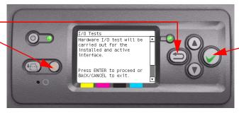
**6** The Printer will get information on the I/O Interfaces. Once the information has been read, the following message will be displayed on the Front Panel. Press any key to continue with the test:
