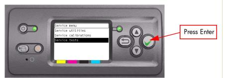
4 In the Service Tests submenu, scroll to "I/O Tests" and press Enter.
