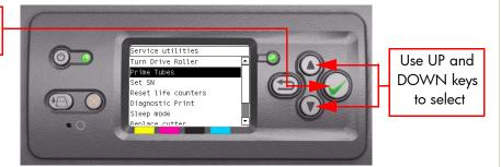
If the printer is not used for 135 seconds, the printer exits out of the Service Utilities Menu and you must repeat the above steps to enter Service Utilities again.
