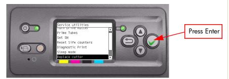
When the following message appears on the front panel, you must select whether you would like to continue with replacing the Cutter by pressing the **Enter** key. Press **Back** or **Cancel** to exit the utility.
