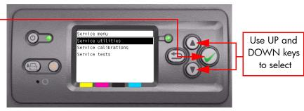
5 Use the **Arrow** keys to scroll through the "Service Utilities" selections and press the **Enter** key to begin a specific operation when the required Service Utility is highlighted.
