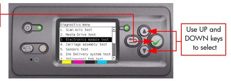
The Service Tests work in a special Mode which does NOT require the full Initialization of the Printer. Therefore it is important that once you have finished with the Service Tests, you MUST power OFF the Printer and Power ON again before trying to print.
