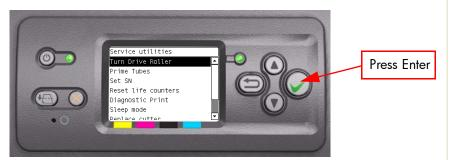
2 The Printer checks to see if media is loaded. If media is loaded, the Front Panel will display the following message. Unload the media and start again from step 1:
