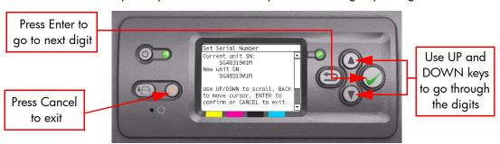
If the Serial Number or the Part Number cannot be read, the Front Panel will display **System Error Code 74:00**. For more information on troubleshooting this error code, refer to Page 2-20.
