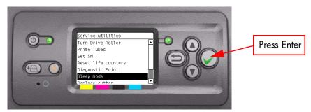
2 When the following message appears on the front panel, use the **Up** and **Down** arrow keys to either disable or enable the sleep mode. Press the **Enter** or **Cancel** key to confirm the selection.
