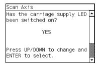
4 Open the Window and check that the Carriage power light is ON (a green light on the carriage PCA). Select Yes or No by using the Up and Down keys and press Enter to confirm your selection.
