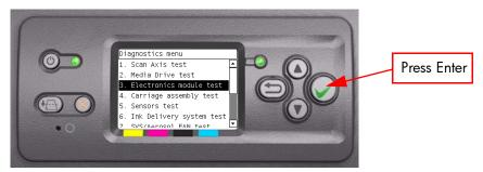
2 A message will appear on the Front Panel asking whether you would like to check the Formatter. Select Yes or No by using the Up and Down keys and press Enter to confirm your selection. If you select No, the printer skips this test and goes to the next one:
