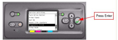
2 You will be given an option to either print the "Image Quality User Plot" or the "Image Quality Service Plot". Use the **Arrow** keys to make the selection and press the **Enter** key to start printing the required Diagnostic Print.
