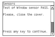
If the Window Sensor fails the test, the Front Panel will display **System Error Code 51:10**. For more information on troubleshooting this error code, refer to Page 2-15. Check also **System Error Code 07:10** (refer to Page 2-6).
