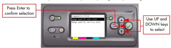
3 Make sure media is loaded, the Pinch Lever is lowered and that the Ink System is correctly installed. Press the **Enter** key to print the Diagnostic Print or press **Back/Cancel** to exit without printing the Diagnostic Print.
