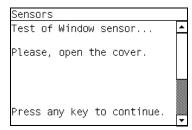
**6** If the Window Sensor passes the test, the following message is displayed on the Front Panel. Close the Window and press any key to continue.
