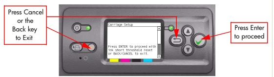
**3** If the Ink Short Thresholds have been reset correctly, the following message will be displayed on the Front Panel. Press any key to exit:
