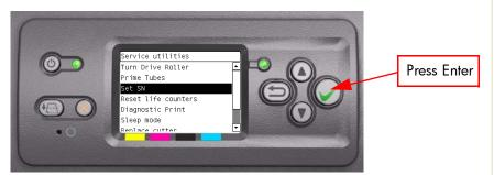
2 The Printer will display the current Serial Number and the new Serial Number of the Printer. Use the Up and Down keys to go through the digits and press the Enter key to go to the next digit. You can press the Cancel key at any time to exit the utility without making any changes.
