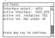
This screens shows which interface is currently installed and active. If a connection is made to the active interface, the "Active int. MAC state" will be displayed as UP, otherwise it will displayed as DOWN.
