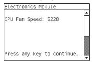
If the CPU Fan Speed is less than 2500, the Front Panel will display **System Error Code 05.1:10**. For more information on troubleshooting this error code, refer to Page 2-5.
