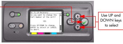
7 If you select **Yes**, the Front Panel will display the new Serial Number and Part Number. Press the **Enter** key to accept.
