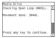
Check that the movement done is **more** than 100 encoder units (in absolute value). If the movement done is **less** than 100 encoder units then open the Window and check for any visible obstacles restricting the movement of the Drive Roller or the Overdrive Assembly.
