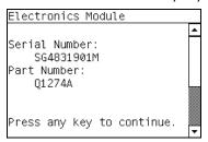
If the Serial Number or the Part Number cannot be read, the Front Panel will display **System Error Code 74:00**. For more information on troubleshooting this error code, refer to Page 2-20.
