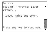
10 If the Media Lever Sensor passes the test, the following message is displayed on the Front Panel. Lower the Media Lever and press any key to continue.
