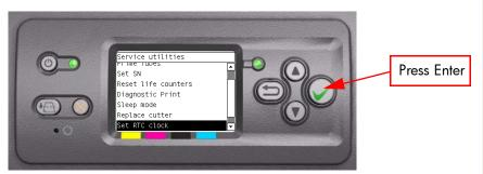
2 The Printer will display the current time and the new time. Use the Up and Down keys to go through the digits and press the Enter key to go to the next digit. You can press the Cancel key at any time to exit the utility without making any changes.
