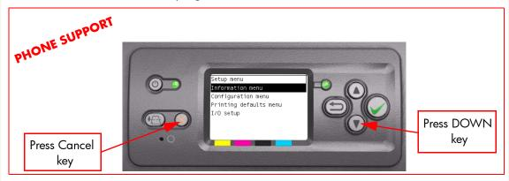
**3** For On-Site Engineers, once inside the "Printer Setup" menu, press the **Up** arrow key and the Cancel key together. You are now in the Service Tools Menu.
