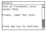
If the Media Lever Sensor fails the test, the Front Panel will display **System Error Code 54:10**. For more information on troubleshooting this error code, refer to Page 2-16. Check also **System Error Code 07:10** (refer to Page 2-6).
