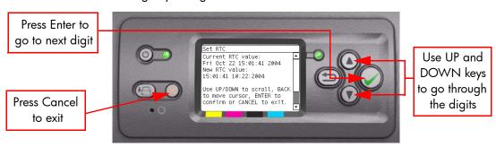
3 Once the new time has been entered, the Front Panel will display the time that you have requested. Press the **Enter** key to confirm the time or the **Cancel** key to exit the utility without making any changes or the **Back** key to modify again.
