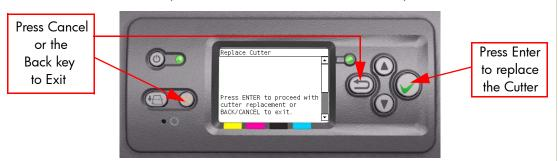
3 The Carriage will move to the Cutter replacement position and the following message will be displayed on the Front Panel. After a few seconds the Printer will begin to shutdown.
