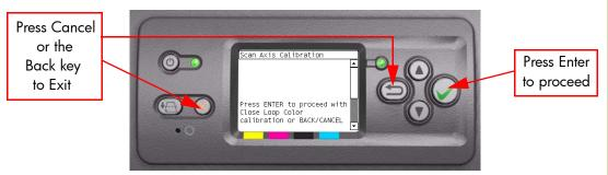
12 Once the Color Calibration is completed, the following message will be displayed on the Front Panel. Press the Enter key to continue.
