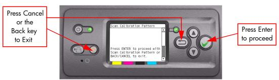
12 A message will appear advising you that you will need to load the Calibration Pattern in to the Printer. Make sure that you rotate the printed pattern 90° clockwise and reload it printed-side down, so that the black arrows go into the printer first. Press the **Enter** key to continue.
