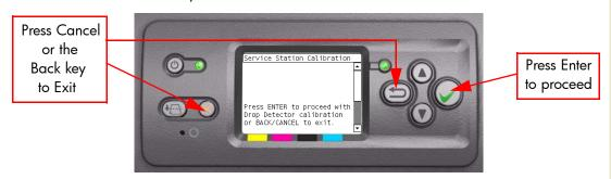
**3** The Printer will start to calibrate the Service Station. Once the Service Station has been calibrated, the results will be displayed on the Front Panel. Press any key on the Front Panel to finish the calibration.
