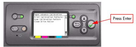
When the following message appears on the front panel, you must select whether you would like to continue with the calibration by pressing the **Enter** key. Press **Back** or **Cancel** to exit the calibration.
