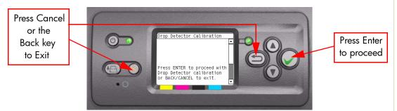
3 The Printer will start to calibrate the Drop Detector. Once the Drop Detector has been calibrated, the results will be displayed on the Front Panel. Press any key on the Front Panel to finish the calibration.
