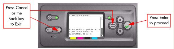
17 The Printer will begin the Drive Roller Cleaning procedure. This could take several minutes during which the following message will be displayed on the Front Panel.
