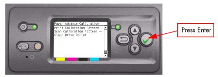
11 When the following message appears on the front panel, you must select whether you would like to continue with the calibration by pressing the **Enter** key. Press **Back** or **Cancel** to exit the calibration.
