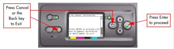
**8** Once the Printhead Alignment is completed, the following message will be displayed on the Front Panel. Press the **Enter** key to continue.
