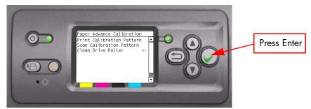
When the following message appears on the front panel, you must select whether you would like to continue with the cleaning of the Drive Roller by pressing the **Enter** key. Press **Back** or **Cancel** to exit the calibration.
