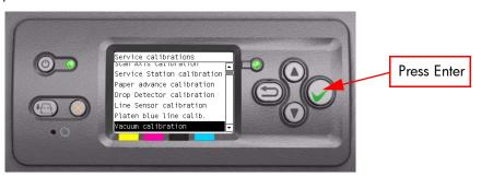
When the following message appears on the front panel, you must select whether you would like to continue with the calibration by pressing the Enter key. Press Back or Cancel to exit the calibration.
