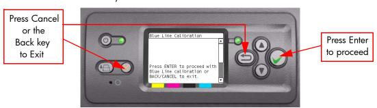
**3** A message will appear on the Front Panel requesting you to raise the Media Lever and to place a sheet of white media on the Print Platen aligned with the Blue Line. Press the **Enter** key to continue once the sheet is in placed.
