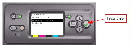
**4** Use the **Arrow** keys to scroll through the "Service Calibrations" selections and press the **Enter** key to begin a specific operation when the required Service Calibration is highlighted.
