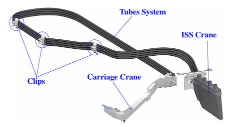
In both ends of the tubes there are fluidic interconnections which are designed to prevent any kind of ink leakage, and minimize the ink on customers as they interact with the system (i.e. when they must replace Ink Cartridges or Printheads).
