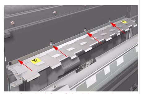
Make sure the Infeed Unit is firmly pushed up against the Printer
