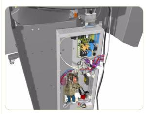
**6.** Remove 3 T-20 screws that secure the Main PCA from the outside.
