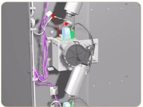
**5.** Disconnect the Cables connected to the Spindle Drive Motor.
