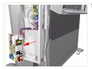
7. Remove the Power Supply Unit.
