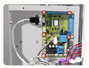
**7.** Remove 6 T-20 screws that secure the Main PCA from the inside.
