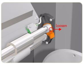
**3.** Loosen 1 screw (Allen key 3 mm) that secures the bushing to the Riding Roller.
