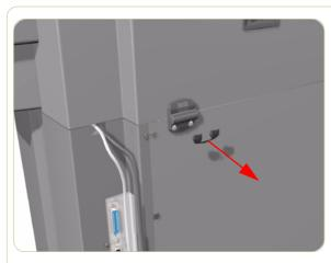
**4.** Remove the screw covers from both sides.
