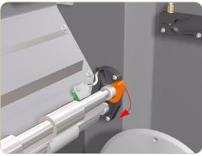
**2.** Lower the Roller Levers on both sides of the Riding Roller.
