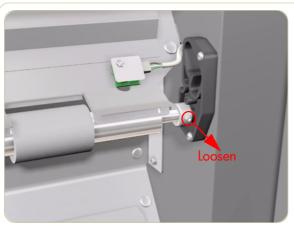
**7.** Loosen 1 screw (Allen key 2.5 mm) that secures the bushing to the Transport Roller on the right hand side (inside).
