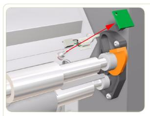
**3.** Disconnect the Cable from the Channel Sensor and remove.
