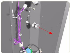
After replacing the Drive Clutches, make sure you reset the counter length for the corresponding roll (e.g. if you replaced the Drive Clutches for Roll 1, reset the partial length counter for Roll 1 to zero). To reset the counter  $\Rightarrow$  Page 1-18.
