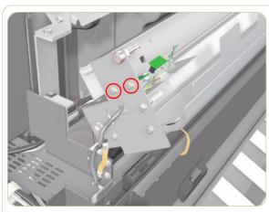
**4.** Remove 2 T-20 screws that secure the Motion Control Sensor.
