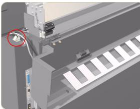
**6.** Release the Cable that is attached to the top of the Right Side Cover.
