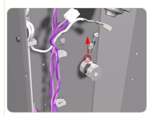
**6.** Remove the inner and outer Drive Clutches and the Transmission Washer together.
