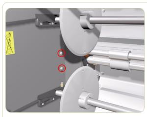
**6.** Remove 2 T-20 screws that secure the Spindle Drive Motor from the inside.
