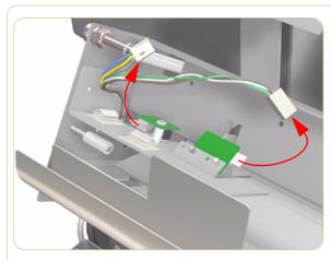
**4.** Disconnect 2 cables from the Motion Control Sensor and release them from the securing clips
