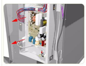
**6.** Remove 5 T-20 screws and 2 Nuts (5.5 mm) that secure the Power Supply Unit.
