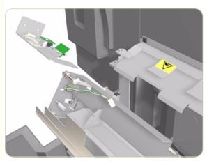
**6.** Remove the Motion Control Sensor.
