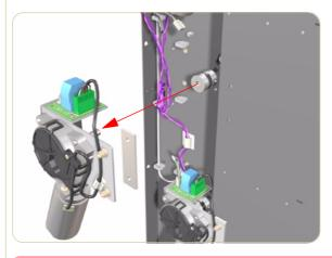
**8.** Remove the Spindle Drive Motor.
