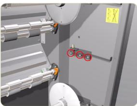
**2.** Remove 3 T-20 screws that secure the Spindle Retainer.
