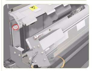
**3.** Remove 2 T-20 screws (one on **each** side of the Motion Control Unit) that secure the Infeed Unit.
