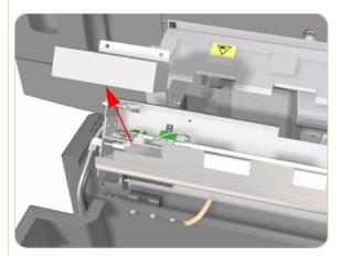
**3.** Remove the Motion Control Unit Sensor Cover.
