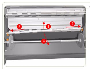
**4.** Raise the Riding Roller first, and then slide it to the right and then remove from the Multi-Roll Feeder.
