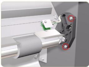
**8.** Remove 2 T-20 screws that secure the right Roller Bearing.
