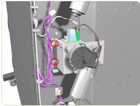
**7.** Remove 2 T-20 screws that secure the Spindle Drive Motor from the outside.
