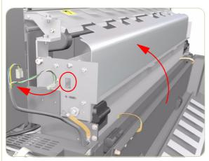
**6.** Close the Motion Control Unit and then pull the 2 motion control sensor cables through the hole in the motion control unit.
