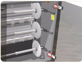
**2.** Loosen 2 screws that secure the Right Door to the Multi-Roll Feeder.
