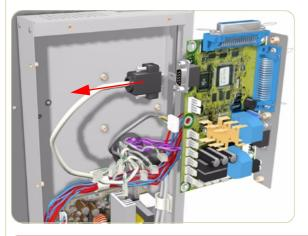
**9.** Disconnect the serial cable from the Main PCA.
