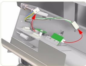
**5.** Disconnect 2 cables from the Motion Control Sensor and release them from the securing clips.
