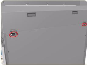
**5.** Remove 4 T-20 screws that secure the Rear Top-Cover.
