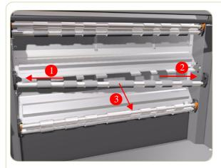
**10.** Slide the Transport Roller first to the left and then remove from the Multi-Roll Feeder.
