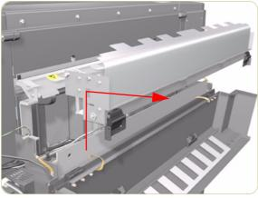
**8.** Remove the Motion Control Unit by lifting it upwards and then towards you.
