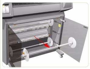
Open both the Left and Right Doors and remove Spindle from the relevant Spindle Retainer.
