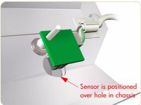
When installing the Motion Control Sensor, make sure you position it as shown in this drawing.
