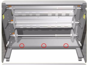
**2.** Remove 3 T-20 screws that secure the Front Bottom Cover to the Multi-Roll Feeder.
