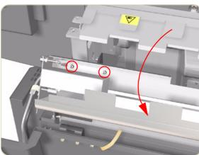
**2.** Open the Motion Control Unit and remove 2 screws from the Sensor Cover.
