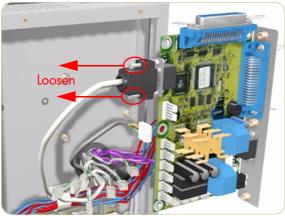
**8.** Remove the Main PCA from the base and loosen 2 screws from the serial cable.
