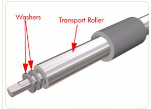
When installing the Transport Roller, make sure you reinstall the same number of washers that you removed from the left hand side of the Transport Roller.
