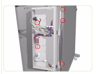
**8.** Remove the Bottom Electronics Cover.
