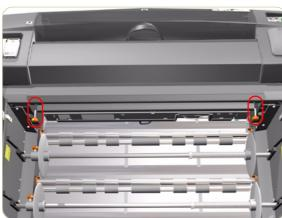
**2.** Remove 2 star screws (**Orange**) that secure the Front Top-Cover to the Multi-Roll Feeder.
