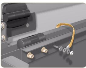
**2.** Remove the Nut and 2 washers that secure the grounding strip to the Rear Top-Cover.
