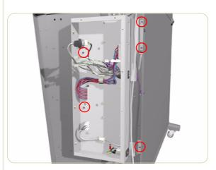
**8.** Remove the Bottom Electronics Cover.
