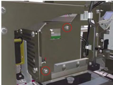
**Be very careful when removing the screws from the Head Cooling Fan Assembly as they can easily fall inside the printer.**
