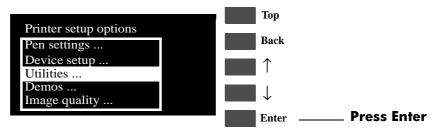
**4** Once inside the "Utilities" menu, use the **Arrow** keys to scroll to the "Test Prints" menu display and press the **Enter** key.
