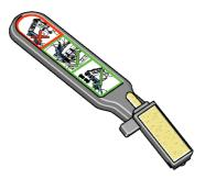
Do not touch, wipe or attempt to clean the printhead nozzles. This can damage the printhead and reduce print quality.
