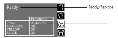
The printer can still operate with a printhead that needs replacing. The front panel will display:
