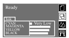
2 Press the ↑ or ↓ key until the front panel displays the ink system menu. Press **Enter.**
