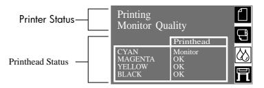
During normal operation the front panel displays the ink levels, however if there is a printhead status message such as: **monitor** for example see page 3-11, *Printhead Status Messages While Printing*, the printhead message will take precedence. This is the case until you replace the printhead. If you need to see the ink levels when they are not being displayed you can use the ink systems menu to check them.
