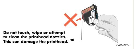
Handle the hp no.80 supplies with care. In particular the printhead, which is a high precision device and must be handled carefully.
