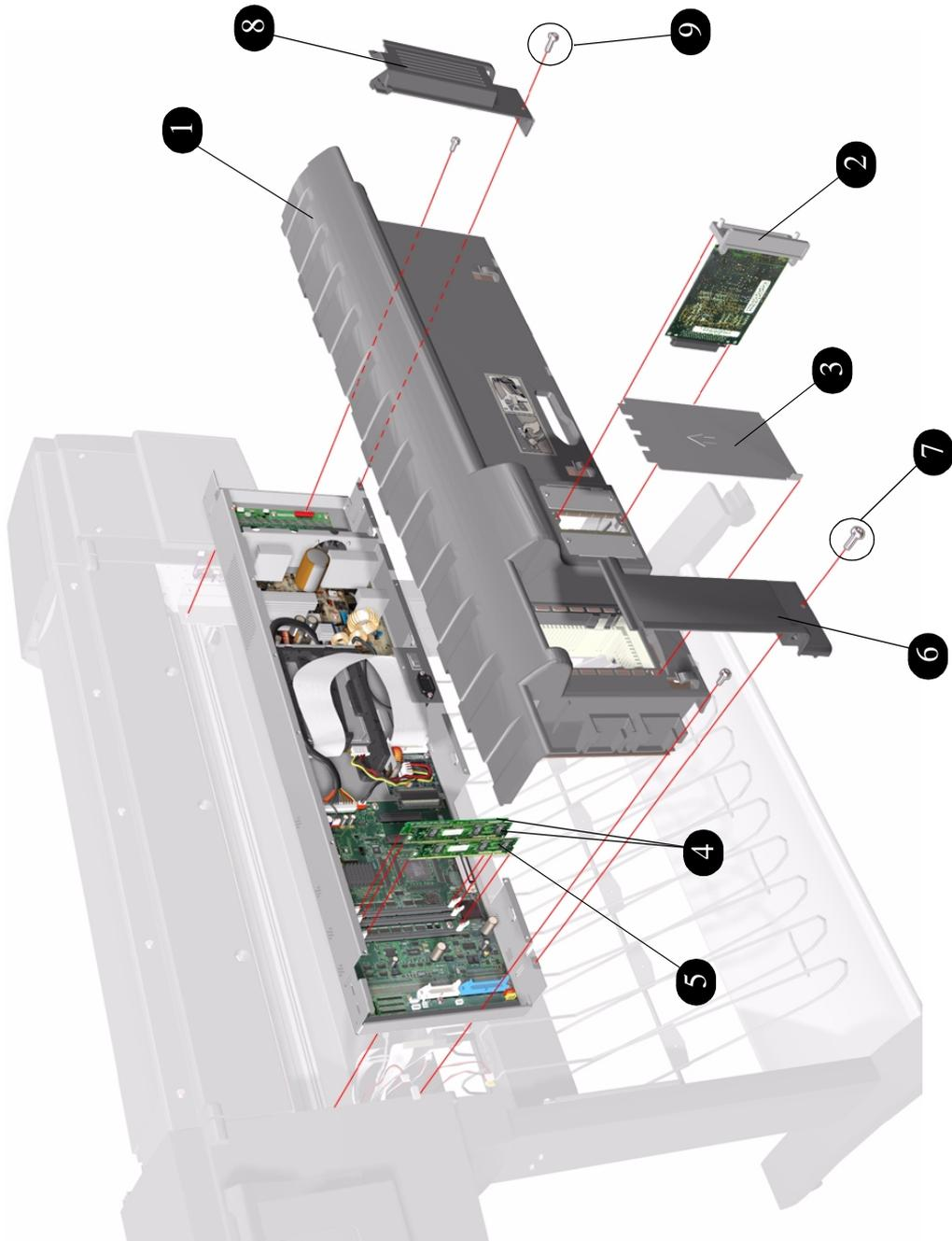
**Figure 6: Electronics Module - External (hp designjet 1050c plus and 1055cm plus)**
