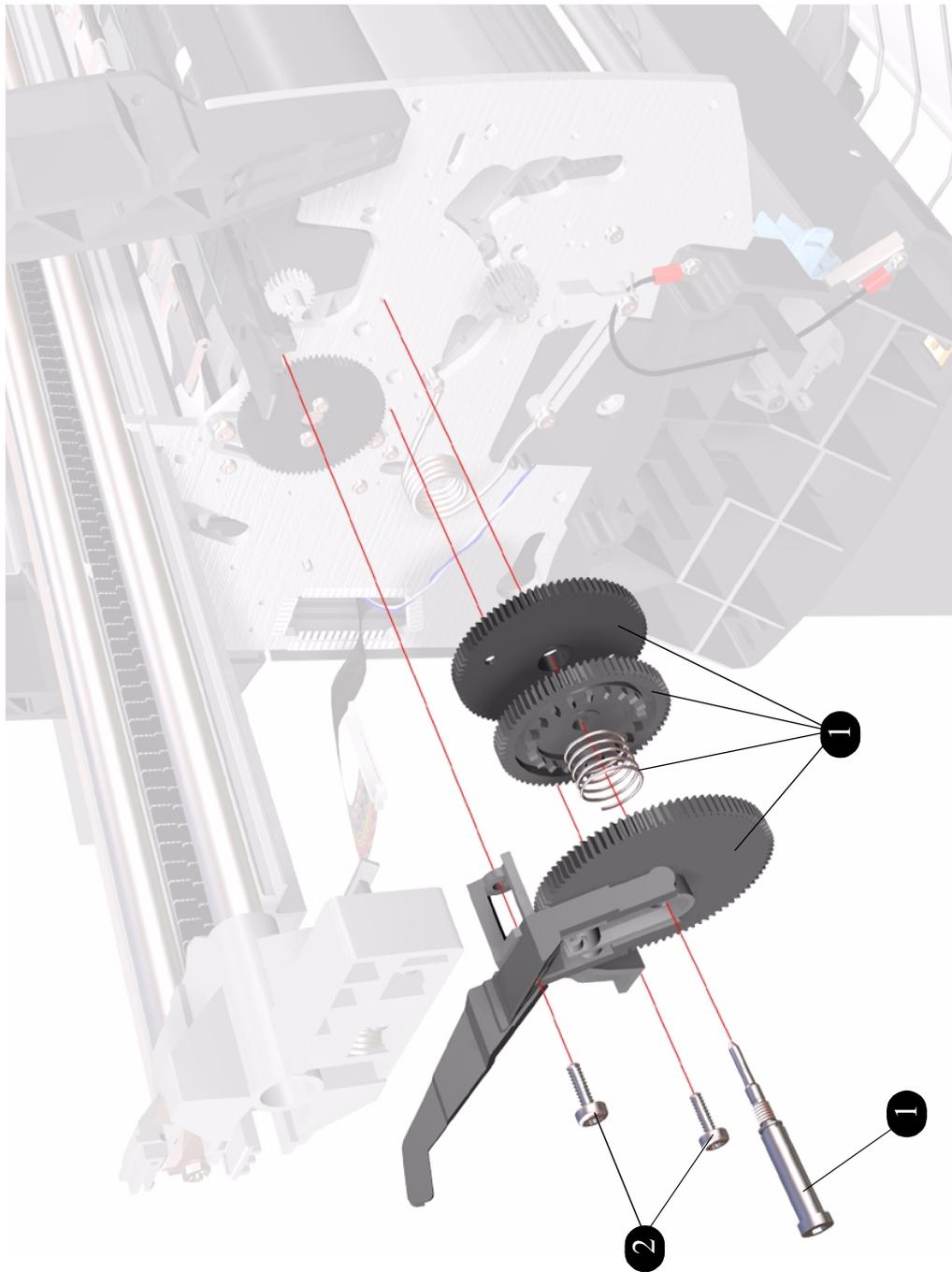
**Figure 11: Clutch Assembly**
