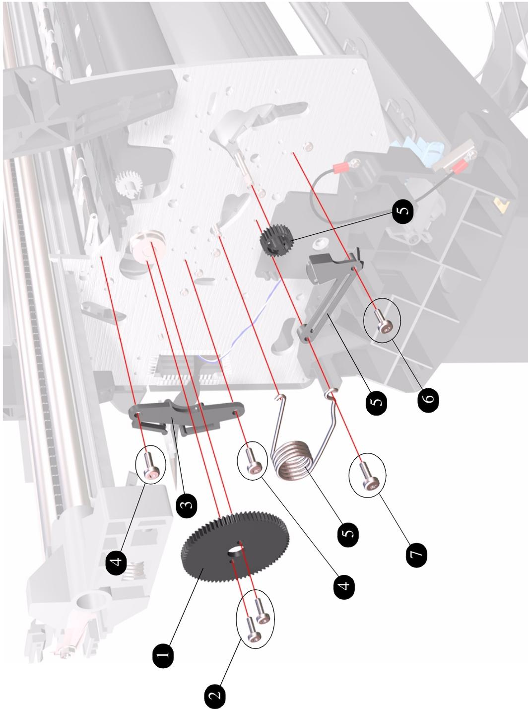
**Figure 14: Drive Roller and ARSS Miscellaneous Parts**
