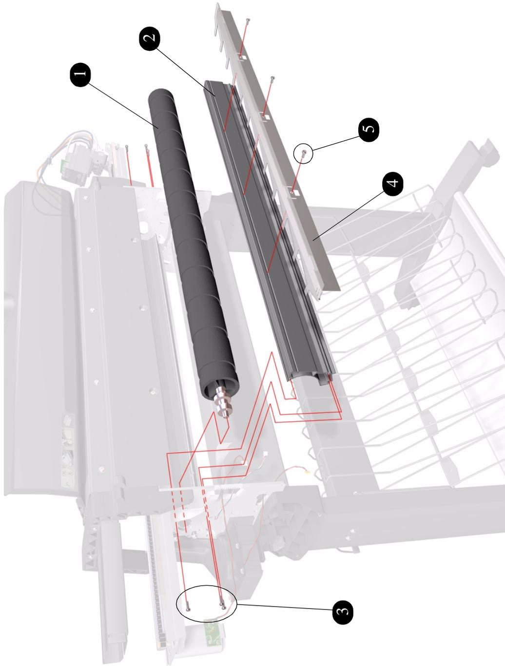
**Figure 17: Drive Roller Assemblies**
