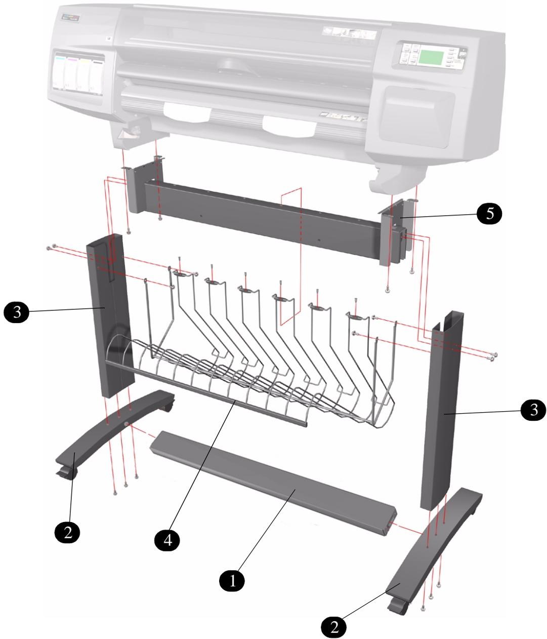
**Figure 1: Printer Support**
