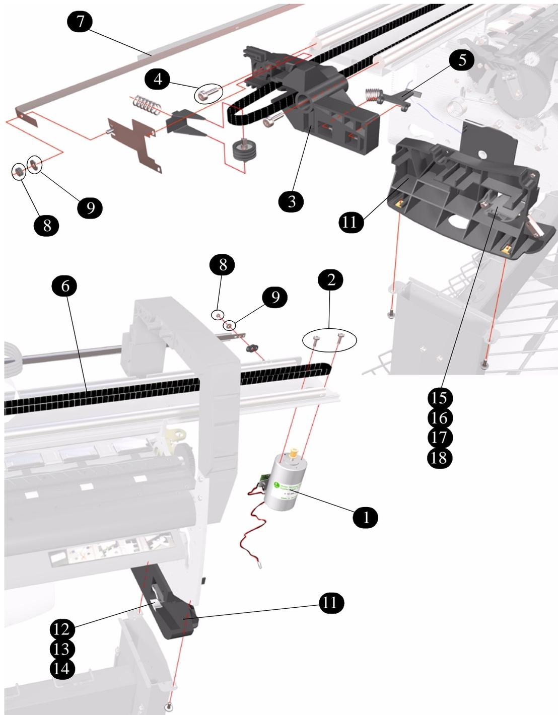
**Figure 13: Scan-Axis Assemblies**
