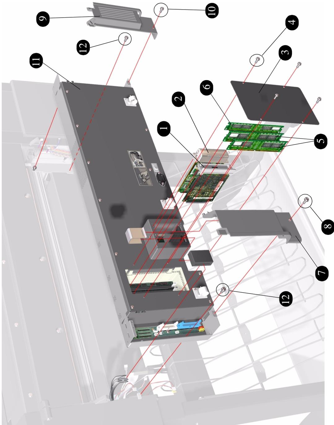
**Figure 4: Electronics Module (hp designjets 1050c/1055cm)**
