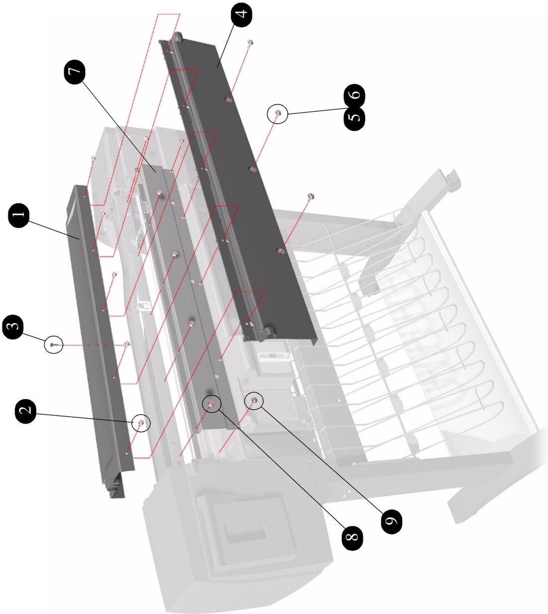
**Figure 3: Rear Covers (hp designjets 1050c plus and 1055cm plus)**
